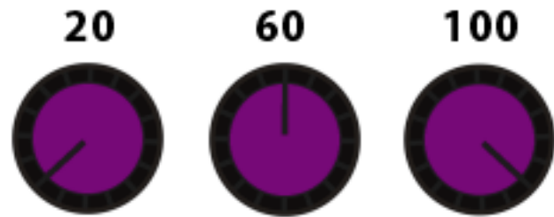
Fig. 5.3 - Potentiometer Min = 20 and Max = 100
