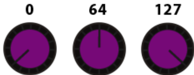
Fig. 5.2 - Potentiometer Min = 0 and Max = 127
