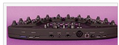
The rear panel of the highest spec JamHub, the TourBus.
